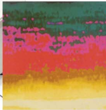
Example of the dramatic heat loss from the surface of a conventional steel griddle.
